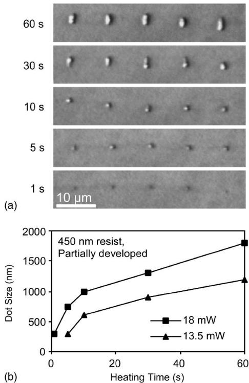
FIG. 3. Dot sizes can be controlled by the heating times as well as heating power. (a) Reduction in size with shorter heating times using a probe biased at 18 mW on 450 nm resist. (b) Dot sizes vs heating time for 18 and 13.5 mW power.
