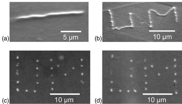
FIG. 5. (a) and (b) Lines of 500 nm width written by patterning successive dots with 200 nm spacing (1 s heating per dot) can be seen after partial development of the photoresist. (c) and (d) Parallel lithography is demonstrated in which two adjacent probes in the eight-probe array simultaneously generate the same pattern.
