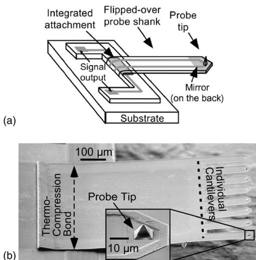
FIG. 2. (a) Schematic of the micromachined single probe, and (b) scanning electron micrograph of the eight-probe array surface micromachined from polyimide on a Si substrate. Thin-film resistors integrated on the tip of the cantilevers allow the individual probes in the array to be heated independently of one another.
