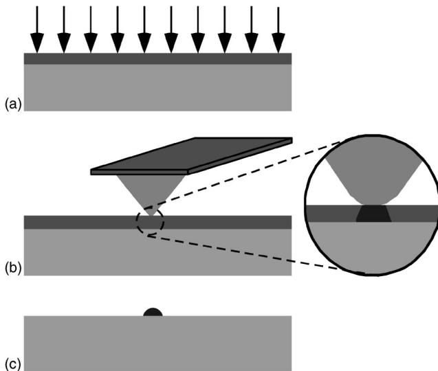
FIG. 1. Process flow for scanning thermal lithography of AZ5214E resist. (a) Flood exposure generates photoacids. (b) Spatially localized thermal crosslinking occurs under the heated probe tip (inset) as a result of the photoacids and elevated temperatures. (c) The insoluble crosslinked region remains after development in TMAH developer.
