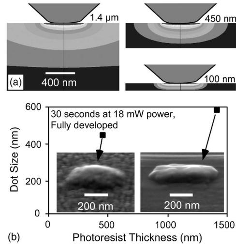
FIG. 4. (a) Finite element simulations with photoresist thicknesses of 1.4  $\mu\text{m}$ , 450 nm, and 100 nm show that the geometry of heat flow becomes vertical as the photoresist is thinned below the diameter of the tip, resulting in smaller features. (b) Dots obtained after fully developing 1400 and 450 nm resists follow the same trend. The roughened surfaces in the micrographs are due to an Au/Pd layers sputtered for scanning electron microscopy.
