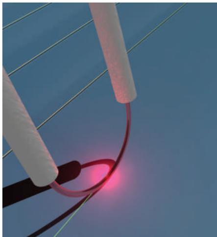
**Figure 1** | Artist's impression of thermochemical lithography. Cacialli and co-workers were able to produce features with line widths as small as 28 nm by scanning a heated wire over a polymer surface<sup>7</sup>. The wire, which is made of platinum and rhodium, has a diameter of 5  $\mu\text{m}$  and is heated by passing a current through it.
