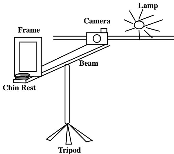
**Figure 1.** A schematic diagram of the experimental setup which is used to snap the images. The subject sits in a chair (not shown) which is positioned in front of the frame.
