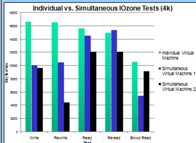
The figure above shows that the simultaneous Virtual Machines always have different performance. The Rewrite and Backward Read tests showed the biggest performance difference.
